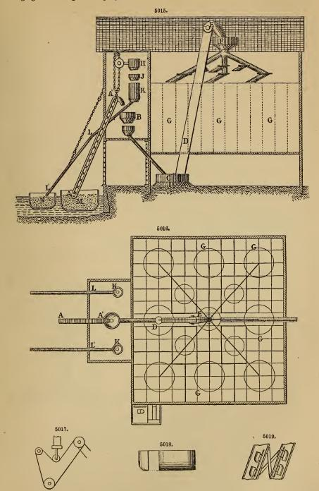
B, receiving and weighing hoppers; C, interior wells; D E, receiving elevator; F, distributing reservoir; G G, bins; H, bolter; J, weighing machine for grain to be reshipped; K, shipping garners; L L', shipping spouts; M, lake boat; N, canal boat. Figs. 5018, 5019, are details of the elevator. All the appliances for unloading, weighing, cleansing, and reloading are here
